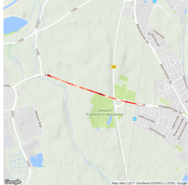
Fig. 4. A east to west drive on the K3535. Red indicates higher IRI, white indicates lower IRI.
